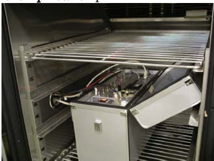
J-chip reader put in test chamber
